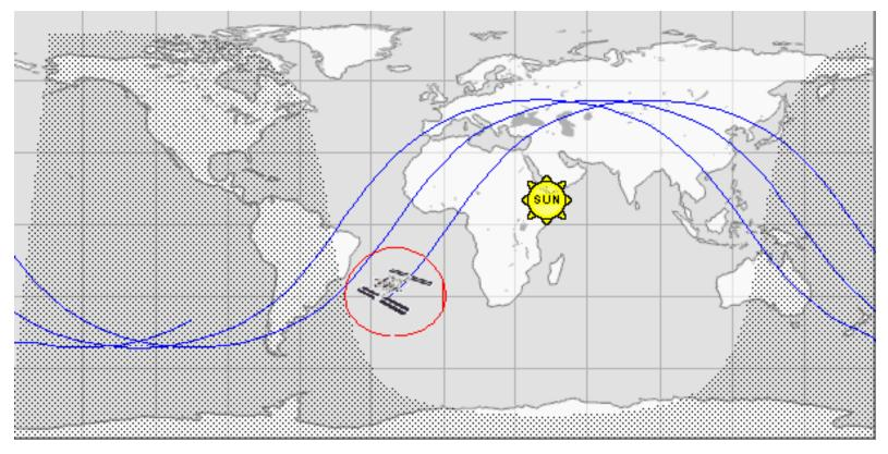
Inclination of 51.6 degrees was chosen to be compatible with Russian launch site, Baykonur, which significantly cut shuttle payload weight.
